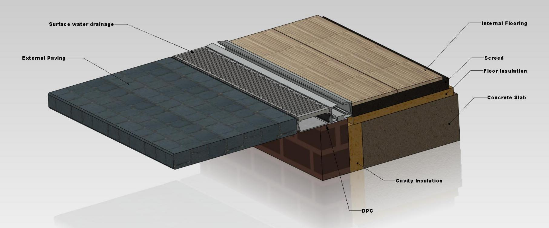
Drawing shows a non weathered threshold without a cill and with internal and external floor finishes at the same level
