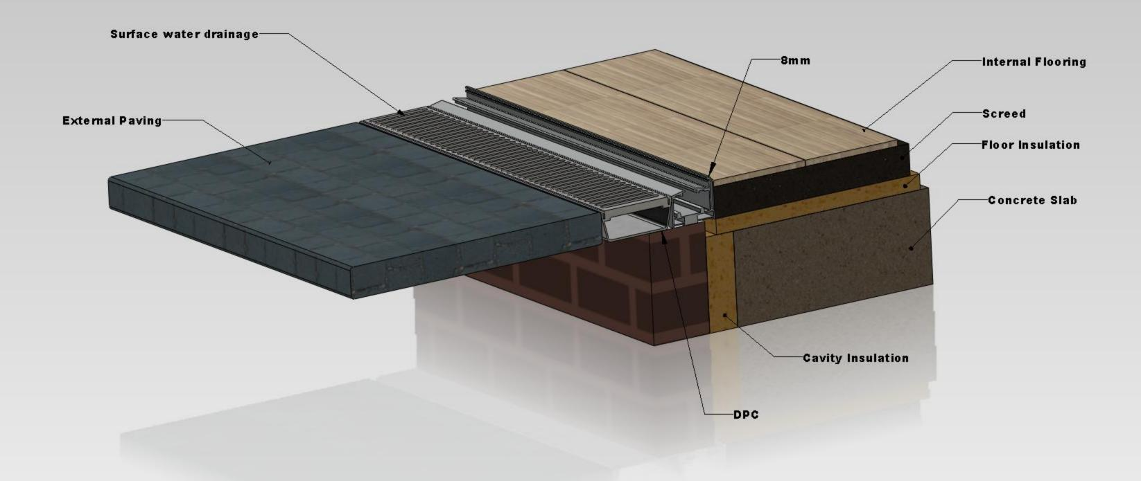
Drawing shows a fully weathered threshold with no cill and virtually flush internal and external floor finishes
