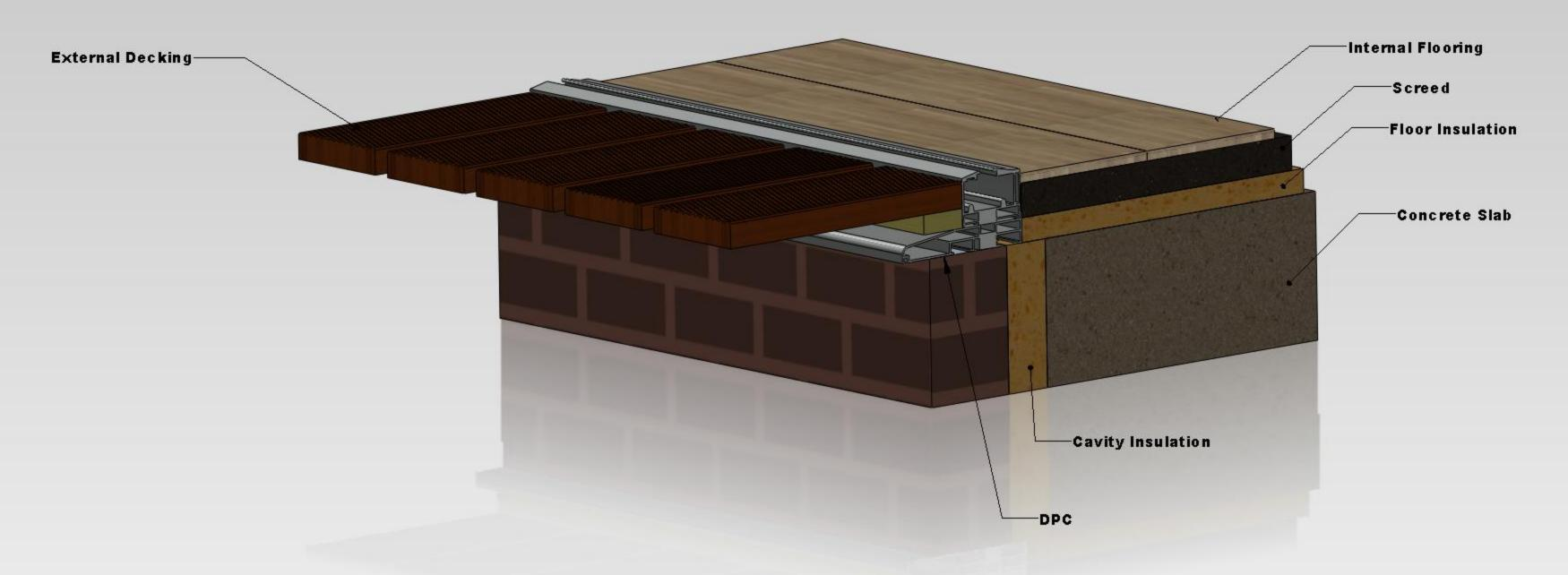
Drawing shows a non weathered threshold with a cill with internal and external floor finishes at the same level
