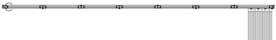
Suitable for apertures 2800mm to 8400mm wide and upto 2500mm tall
