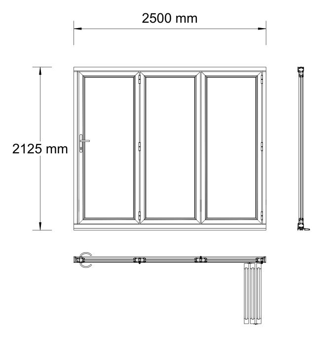
Suitable for apertures 1200mm to 3600mm wide and upto 2500mm tall
