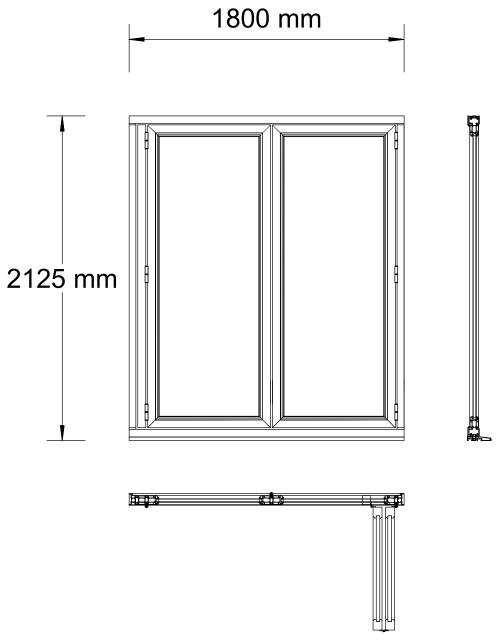
Suitable for apertures 1400mm to 2400mm wide and upto 2500mm tall
