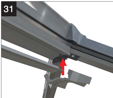
Fit internal ridge claddings. Fit internal ridge hub end cover by flexing rear around ridge.
