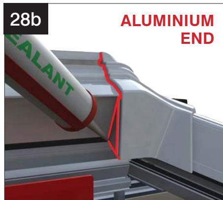
Seal along the ridge baffle where it meets the glazing and over any bar where it meets the ridge.
